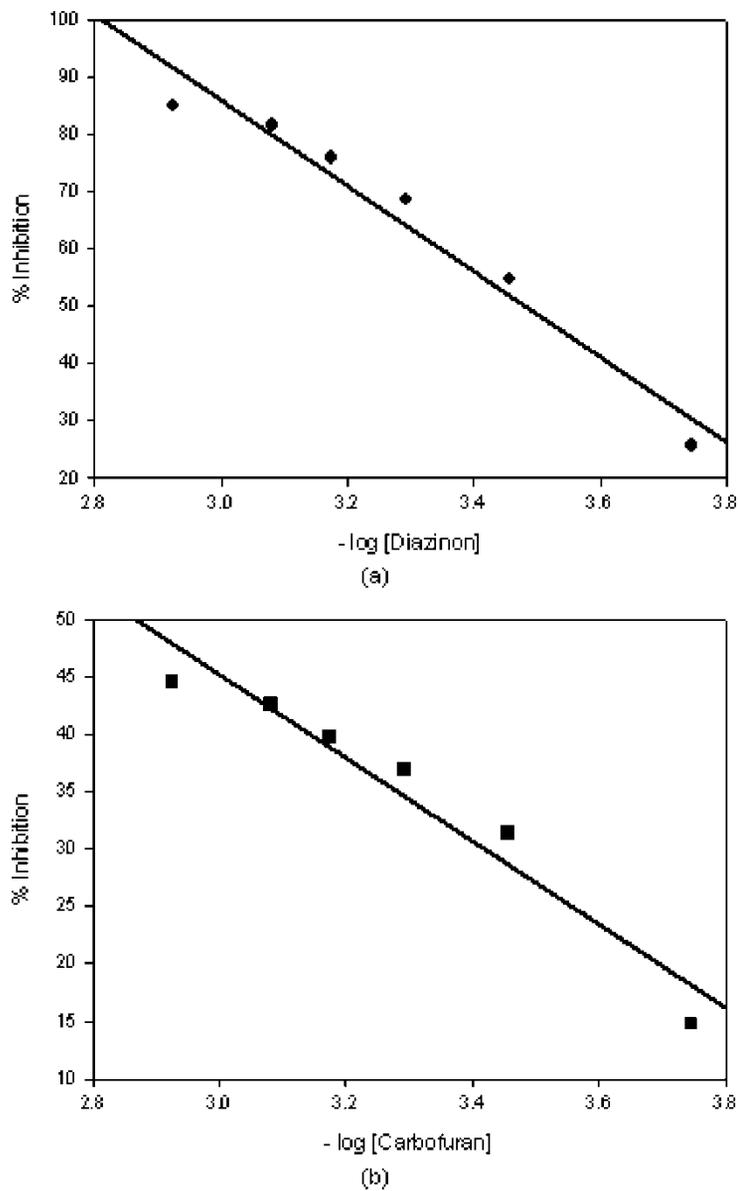
**Figure 9.** The percentage inhibition plot of (a) diazinon and (b) carbofuran for Au/MBT/POMA-PSSA/AChE biosensor in 1.10 mM acetylcholine (0.1 M phosphate buffer, KCl, pH 7.2).
