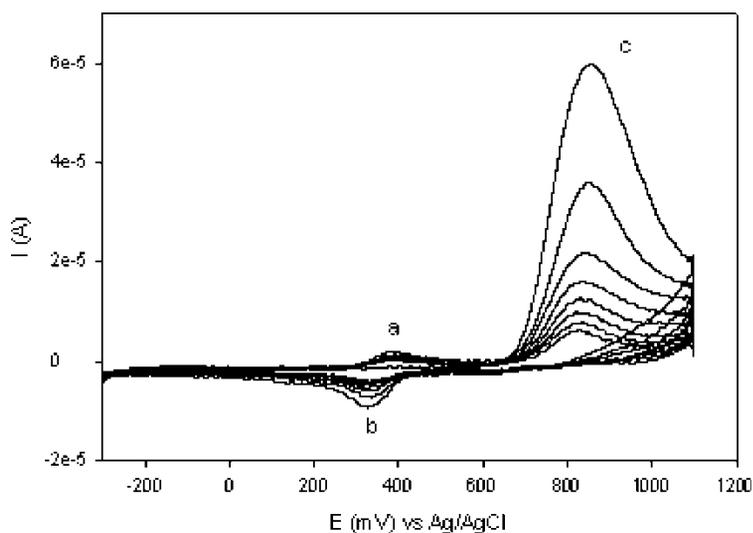
**Figure 3.** Electrosynthesis of POMA-PSSA film in 1 M HCl on Au/MBT-SAM electrode at 20 mV/s from -500 to +1100 mV.
