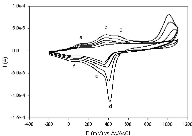
**Figure 2.** Electrodeposition of PDMA-PSSA film in 1 M HCl on Au/MBT-SAM electrode at  $40 \text{ mV/s}$  from  $-200$  to  $+1100 \text{ mV}$ .
