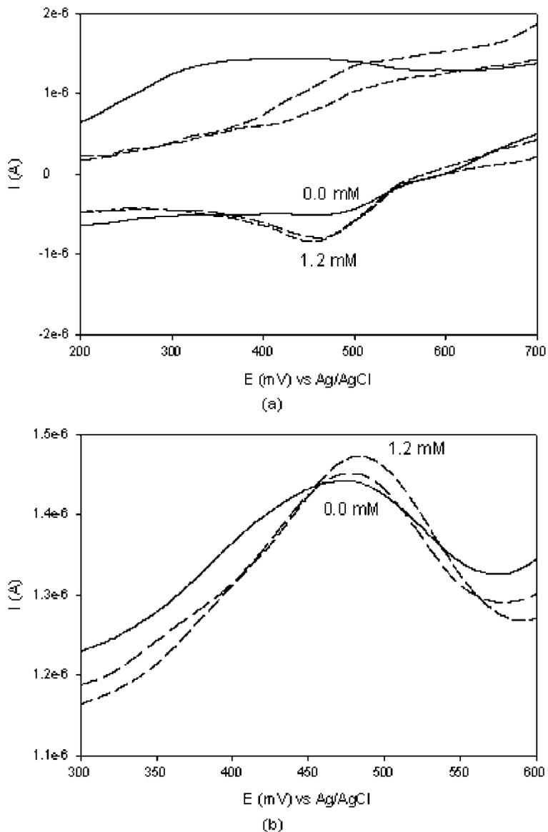
**Figure 5.** (a) Cyclic voltammogrammetric (10 mV/s) and (b) differential pulse voltammogrammetric (5 Hz) responses of Au/MBT/POMA-PSSA polymer film to acetic acid.
