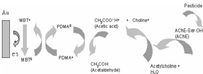
**Figure 4.** A schematic representation of the Au/MBT/PDMA-PSSA/AChE biosensor reaction occurring at the gold electrode, with the pesticide inhibitor effect also indicated.
