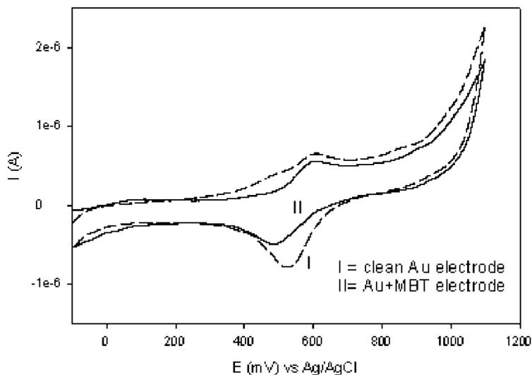
**Figure 1.** Cyclic voltammograms of (I) clean Au electrode and (II) Au/MBT-self-assembled monolayer in 0.1 M phosphate buffer (pH 7.2), from  $-100$  mV to  $+1100$  mV at a scan rate of  $10$  mV/s.
