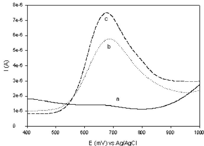
**Figure 7.** Square wave voltammograms of Au/MBT/PDMA-PSSA/AChE biosensor to acetylcholine in 0.1 M phosphate buffer, KCl (pH 7.2), with the potential scanned between +400 to +1000 mV at a frequency of 5 Hz.
