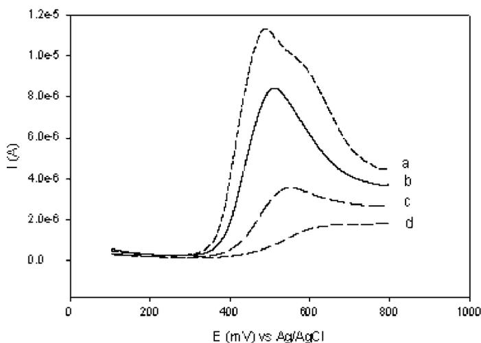
**Figure 8.** Square wave voltammograms of Au/MBT/POMA-PSSA/AChE biosensor responses to diazinon in 1.10 mM acetylcholine (0.1 M phosphate buffer, KCl, pH 7.2) at a frequency of 5 Hz.
