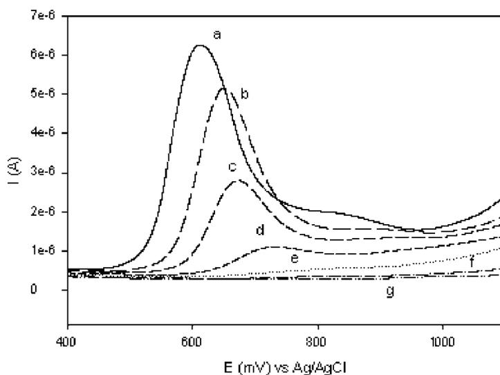
**Figure 10.** Differential pulse voltammetric responses of Au/MBT/POMA-PSSA/AChE biosensor to carbofuran in (a) 1.10 mM acetylcholine alone; and 1.10 mM acetylcholine plus (b) 0.22 ppb, (c) 0.65 ppb, (d) 1.03 ppb, (e) 1.15 ppb, (f) 1.17 ppb, and (g) 1.19 ppb. Experimental conditions are 0.1 M phosphate buffer, KCl, pH 7.2 at a frequency of 5 Hz.
