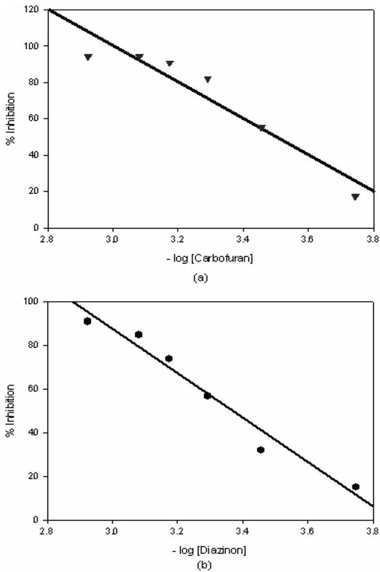
**Figure 11.** The inhibition plot of percentage inhibition vs.  $-\log$  (Carbofuran) pesticide concentration in (a) and vs.  $-\log$  (Diazinon) in (b) as determined with the Au/MBT/PDMA-PSSA/AChE/ACh biosensor in 0.1M phosphate buffer, KCl (pH 7.2) solution.
