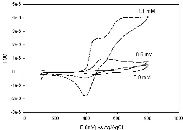
**Figure 6.** Cyclic voltammetric responses of Au/MBT/POMA-PSSA/AChE biosensor to acetylcholine in 0.1 M phosphate buffer, KCl (pH 7.2), with the potential scanned between +200 to +800 mV at a scan rate of 5 mV/s.
