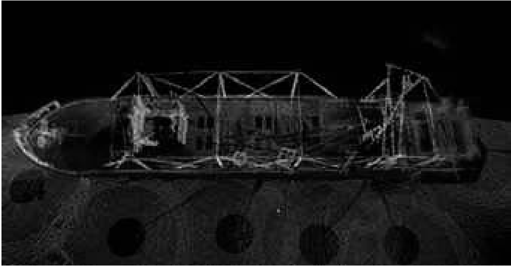
Figure 5: 3D image of the A.J. Goddard (1901) wreck, captured using BlueView technology. This wreck is on the seabed (Dean, 2010).
