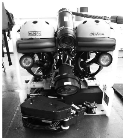
Plate 8: A small research ROV fitted with cameras, lights and a manipulator arm for sample collection (image by Albrecht Götz).
