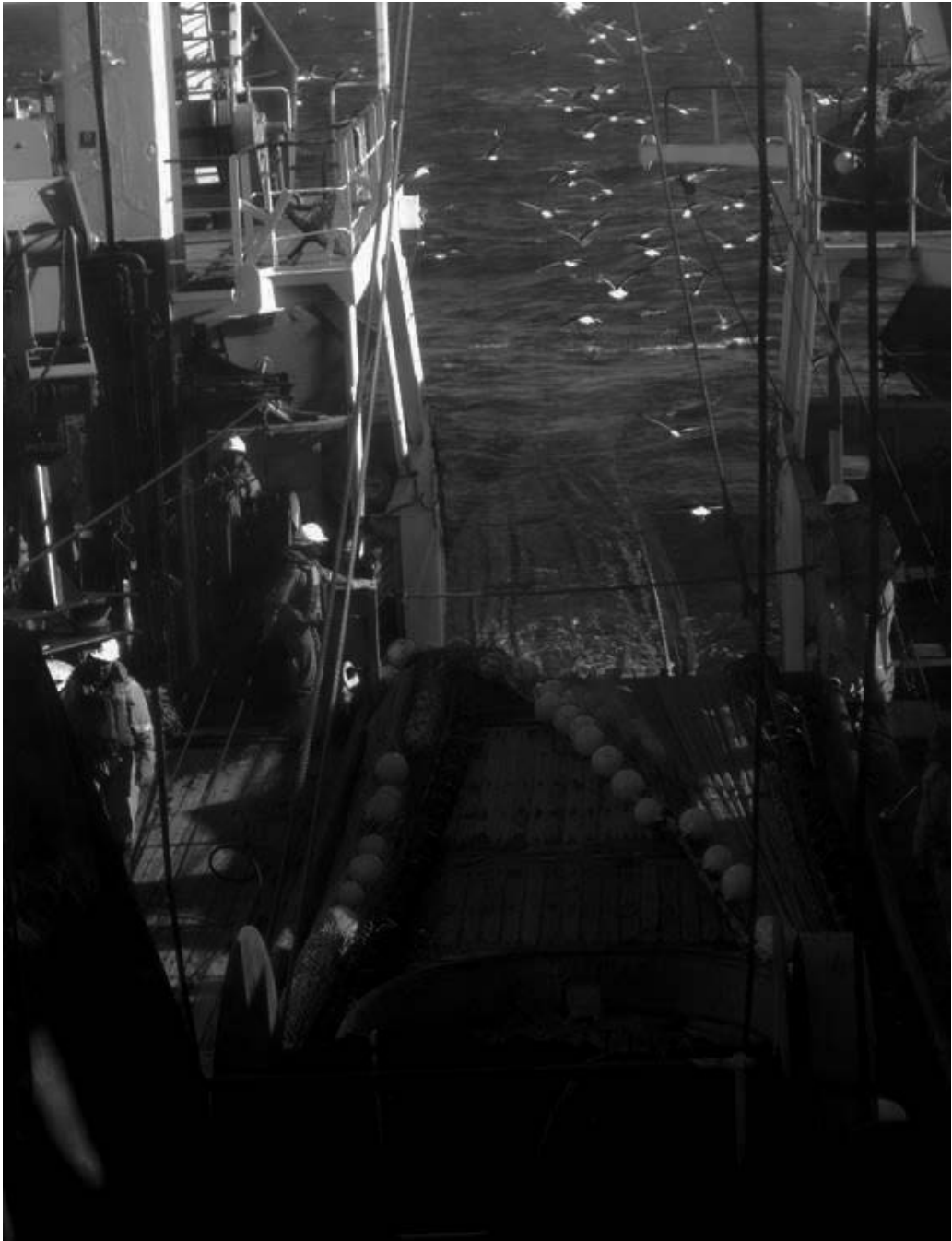
Plate 2: A midwater trawl on FRS Africana retrieving a catch of pelagic fish taken from a school detected by the echo sounder. The arrival of birds during retrieval is usually indicative of other schools in the area and of a good catch.
