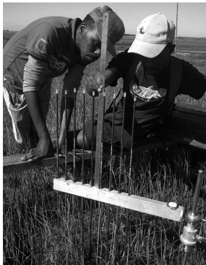
Plate 3: RSET measurements taken by SAEON students in the Swartkops Estuary in 2014 (Image by Tommy Bornman).
