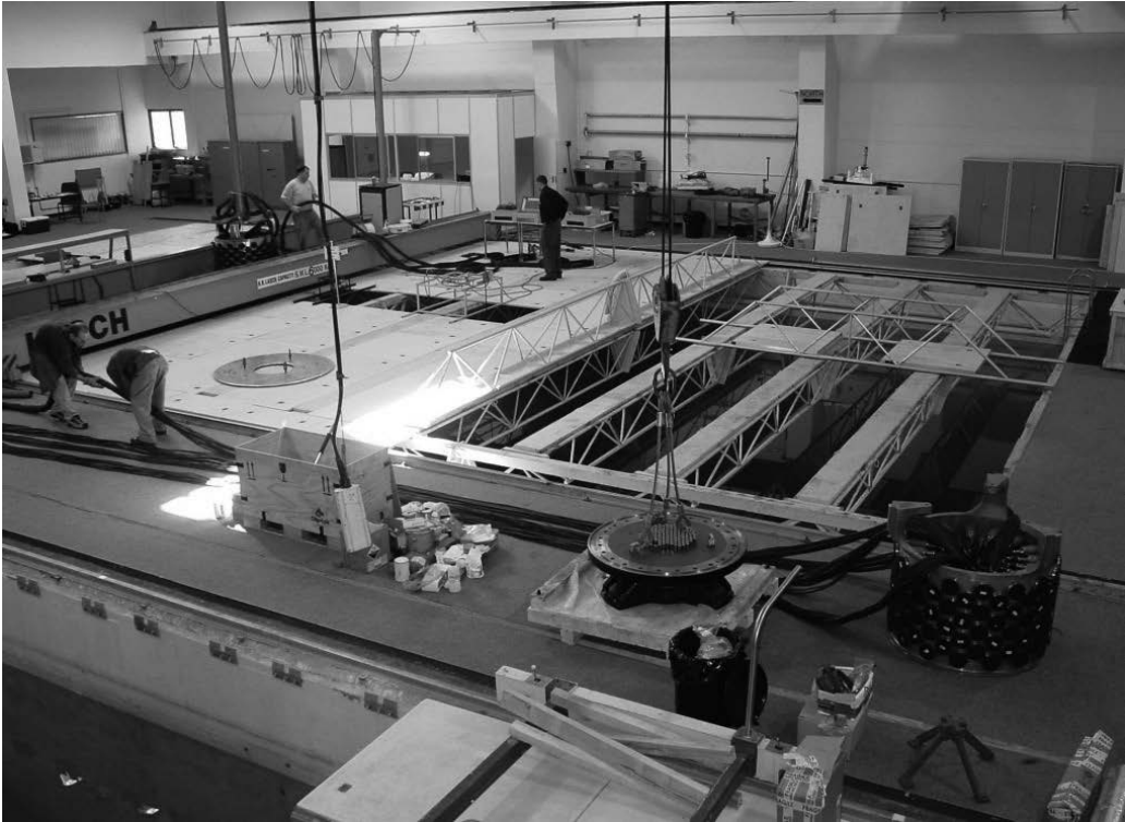
Plate 21: Transducer testing and calibration facility.
