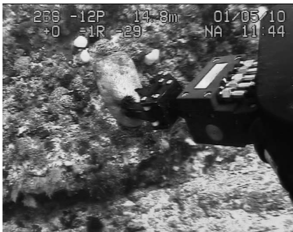
Plate 9: Specimens of benthic growth being collected with an ROV's manipulator arm (image by SAIAB).
